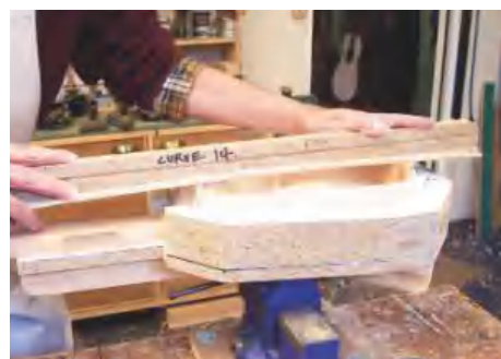
STEP 29. Sanding the 3mm lift
